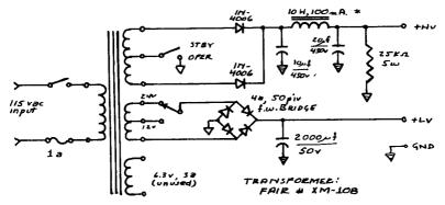
\* ALTERNATELY, USE CHOKE FROM INSIDE RECEIVER UNDER DYNAMOTOR MOUNT.
